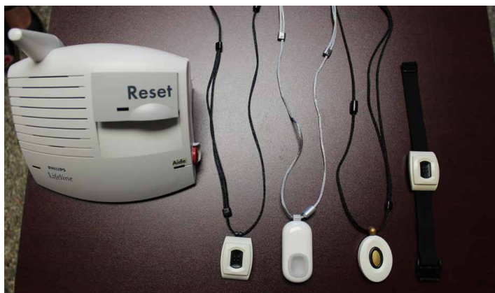
HomeSafe equipment. Some necklaces offer an AutoAlert, which activates a call if a client falls or is in any way unable to press their button.
